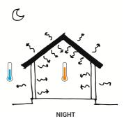
Radiates it in night increasing the internal temperature
