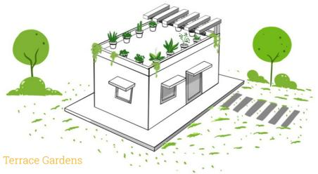
Terrace gardens reduce overall heat absorption of buildings and insulate the building against heat & cold. They provide shade by breaking the solar radiations, improves air quality and cools the surrounding air.
